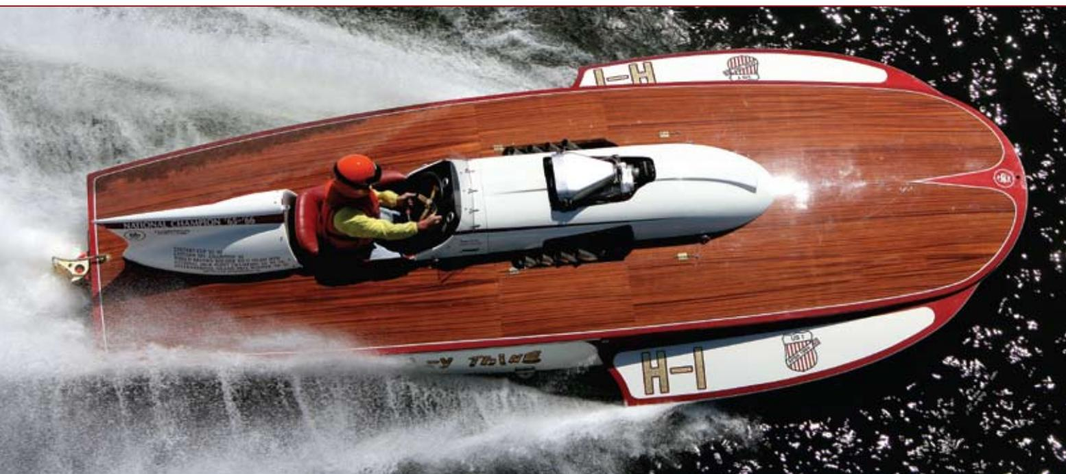
up the way it is today. According to David, “We replaced the trim tab, propeller, and tuned up the 350 engine which was now the powerplant.”
